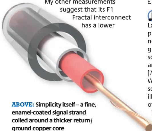
**ABOVE:** Simplicity itself – a fine, enamel-coated signal strand coiled around a thicker return/ground copper core
